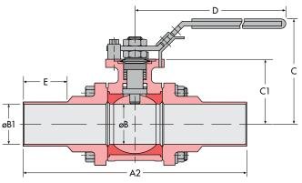
**Extended Tube End Connections**Model S7700
