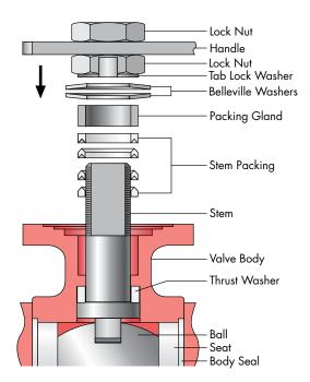
**Stem Seals** The Thrust Washer provides the primary seal while the live loaded Stem Packing creates a multiple secondary seal between the stem and body. The stem packing is also composed of PTFE providing high purity protection and high cycle life. This dual stem seal arrangement is a Flow-Tek exclusive.
