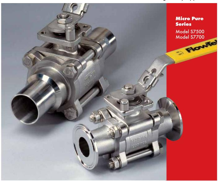
Flow-Tek's Micro Pure Series ball valves have been specifically designed to meet the requirements of high purity applications in accordance with ASME BPEa specification. All valve bodies are investment cast CF3M (316L) Stainless Steel with an internal surface finish of 15 Ra with 20 Ra maximum per SFV-1. Other grades of surface finishes, including electropolishing are available. Cavity fillers and purge ports are also available upon request.
